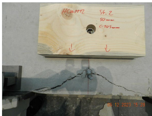
Fig. 4.2: Concrete edge failure, Example c_1 = 105 mm, t_m = 50 mm
