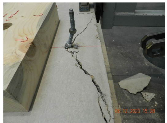
Fig. 4.2: Concrete edge failure, Example c_1 = 105 mm, t_m = 50 mm
