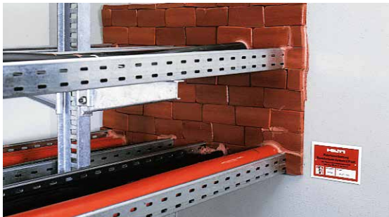
Fig. 8: Preformed firestop block, Hilti CFS-BL Firestop Block used for sealing large openings with multiple through penetrations. The firestop block should be stacked with staggered seams within the opening
