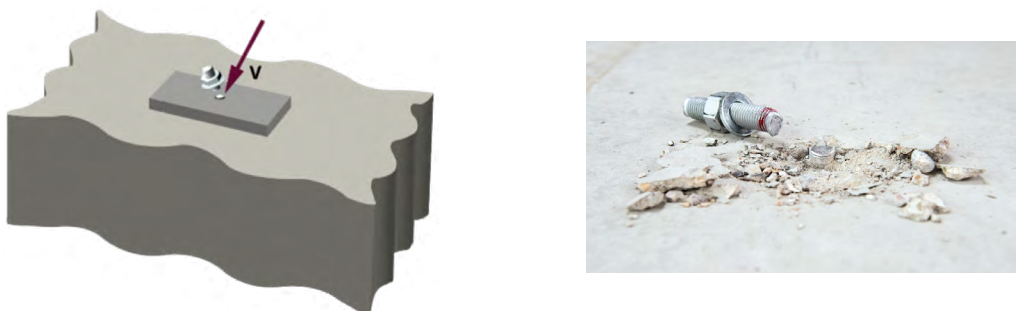
a) Failure without lever arm
