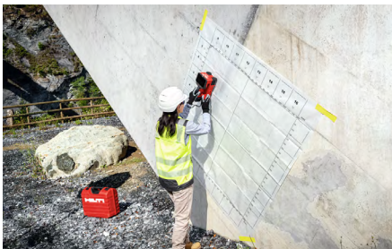
a) Scanning for ferrous objects
