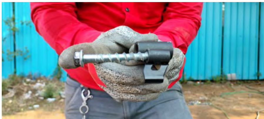
b) Hilti anchor with re-usable gauge
