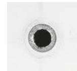
Shiny ring around the bore hole
