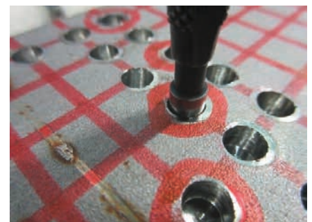
Testing of pilot hole quality
