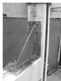
Fig. 7: Steel haunches for local strengthening of beam-to-column reinforced concrete frame and effect of flexural deformation of beam and column on the force distribution on the anchorage [9]
