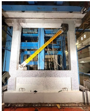
Fig. 6: Diagonal steel brace with its connection and deformed concrete frame
