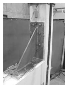
Fig. 7: Steel haunches for local strengthening of beam-to-column reinforced concrete frame and effect of flexural deformation of beam and column on the force distribution on the anchorage [9]
