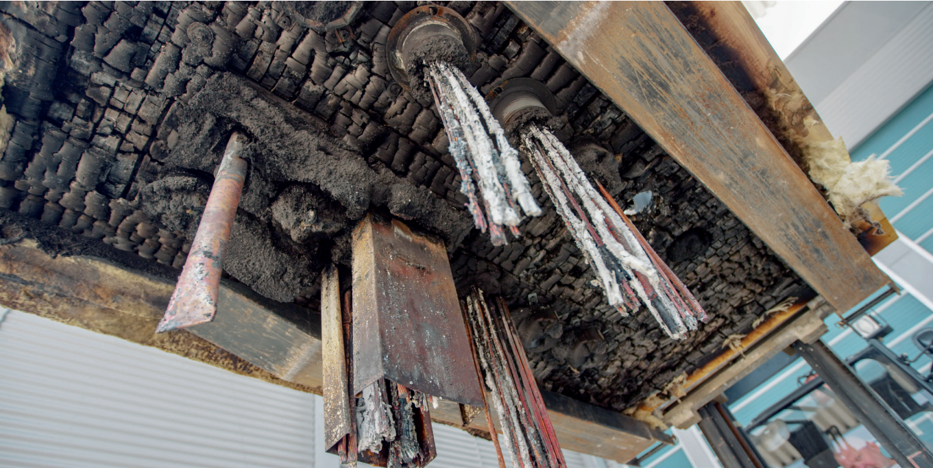
Cross-laminated timber test specimen after a fire resistance test according to EN1366-3
